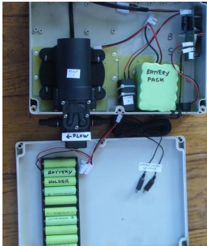
Turn the unit on to number 3, **IF** there is charge in the batteries the pump will start to run after about 5 seconds and the red light will stay on. If the pump stops check the light for the following
