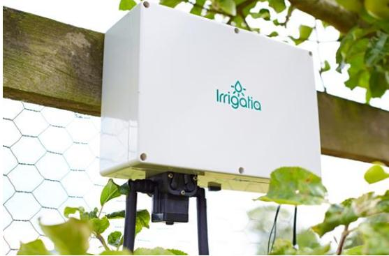
Mount the controller close to the water source and preferably low down so that the pump inlet is below the water line in the tank. The plastic case is weather resistant but can be mounted inside if desired. The solar panel should be mounted, facing the midday sun within 5m of the controller's location. It is easy to disconnect the solar panel lead from the control circuit inside the controller if it needs routing through holes, though re-connecting it may need needle
